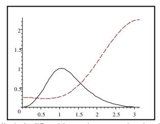
The dashed line is the differential scattering cross section, the solid line is the polarization. The polarization peaks at  $\theta = \pi/3$ . The scattering peaks at  $\theta = \pi$  (backward scattering) and is minimum at  $\theta = \pi/5$ .
